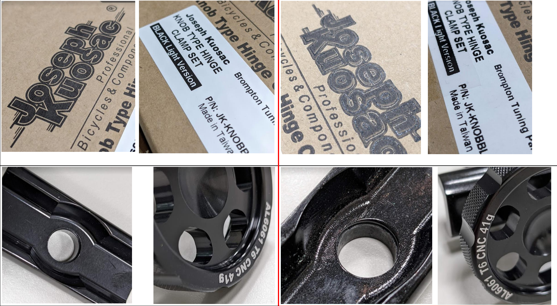
The printing, fonts, laser etching and machining quality are all failed.
